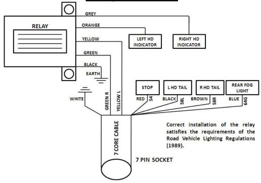
The rear fitting sensor is designed to work in conjunction with a combined hazard warning and indicator flashing unit. Before commencing the fitting ensure the vehicle is parked safely off the road with handbrake on and remove the relevant fuse on the vehicle.
